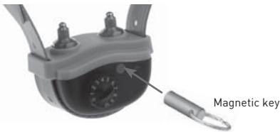
Diagram 3 Activate/deactivate the collar with the magnetic key
